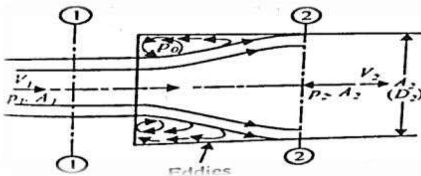
Consider a liquid flowing through a pipe. Due to sudden enlargement in diameter from  $d_1$  to  $d_2$ , the liquid flowing from smaller pipe is not able to follow the sudden change of boundary and turbulent eddies are generated as shown in the figure resulting in loss of head. This head loss due to sudden enlargement is given by  $h_e = (V_1 - V_2)^2 / 2g$
