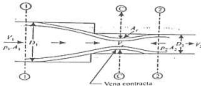
Water is flowing from large diameter pipe to smaller diameter pipe as shown in figure. The loss of head due to sudden contraction is actually due to sudden enlargement from vena-contracta
